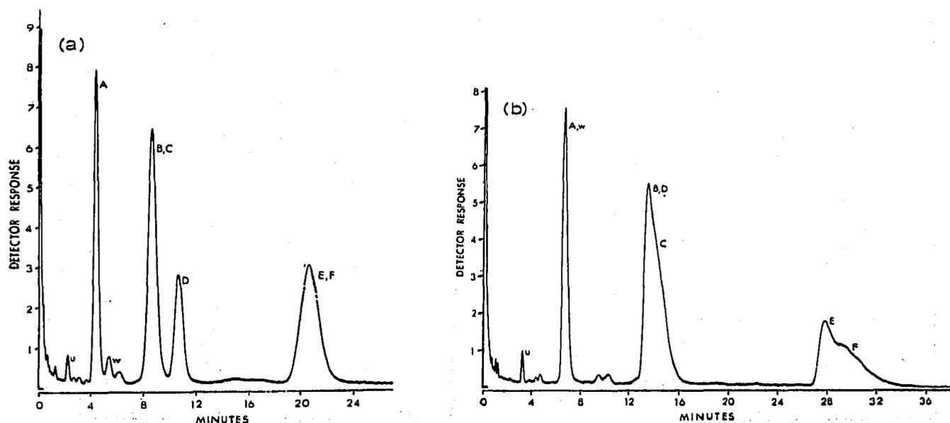
Fig. 3. Typical separations of mixed alkyl ether and monoglyceride TMS ether derivatives on (a) semi-polar XE-60 185° and (b) polar DEGS 200° liquid phases. Peaks identified as alkyl ethers: u = C<sub>14</sub>:0; A = C<sub>16</sub>:0; B = C<sub>18</sub>:0; C = C<sub>18</sub>:1 and monoglycerides: w = C<sub>14</sub>:0; D = C<sub>16</sub>:0; E = C<sub>18</sub>:0; F = C<sub>18</sub>:1.
