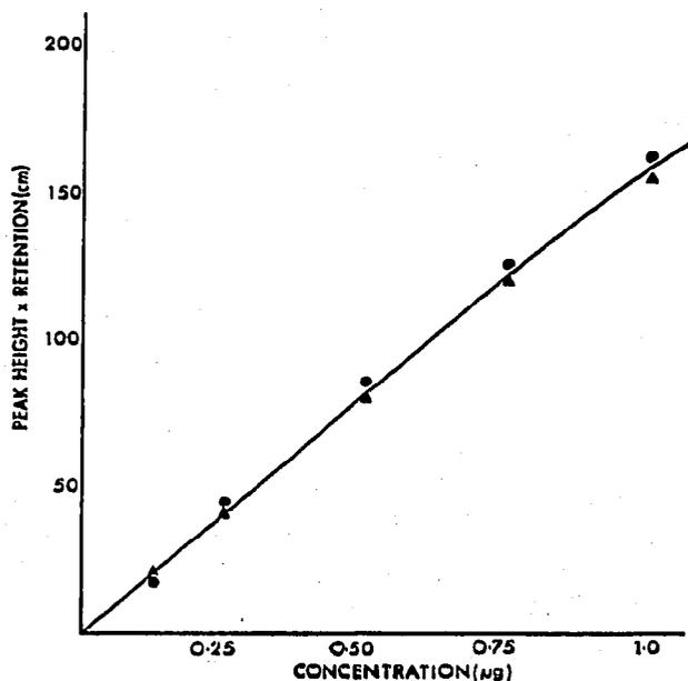
Fig. 5. Plot of concentration ( $\mu$ g) against peak height  $\times$  retention (cm) for C<sub>16</sub>:<sub>0</sub> alkyl ether ( $\blacktriangle$ ) and C<sub>16</sub>:<sub>0</sub> monoglyceride ( $\bullet$ ) TMS ether derivatives. Lipids were chromatographed in pyridine.
