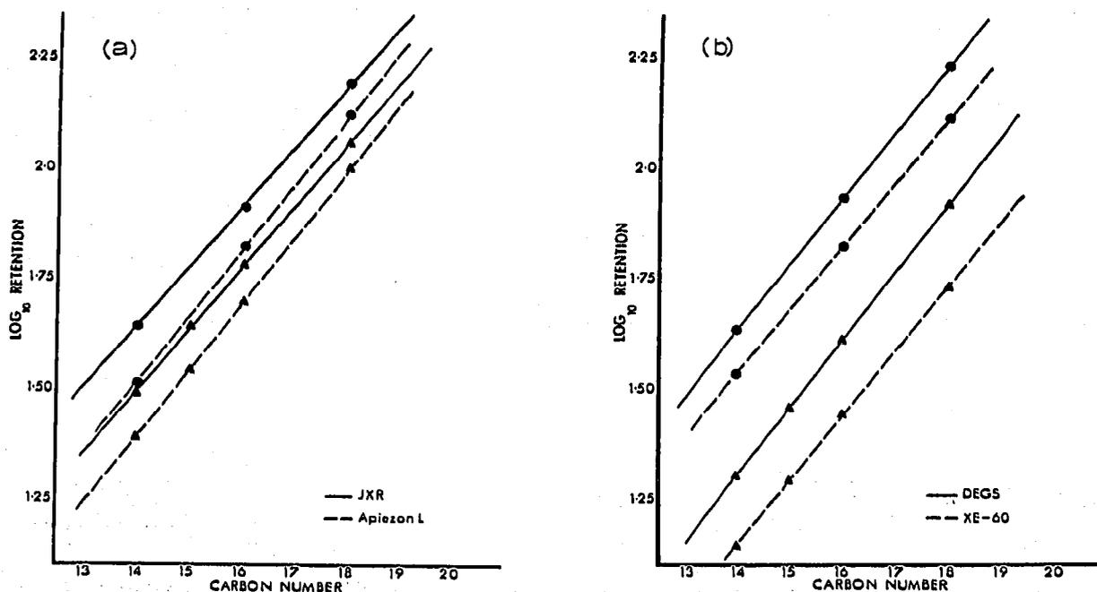
Fig. 4. Plot of  $\log_{10}$  retention against carbon number for individual alkyl ethers ( $\blacktriangle$ ) and monoglyceride ( $\bullet$ ) TMS ether derivatives on (a) non-polar liquid phases and (b) semi-polar and polar liquid phases.
