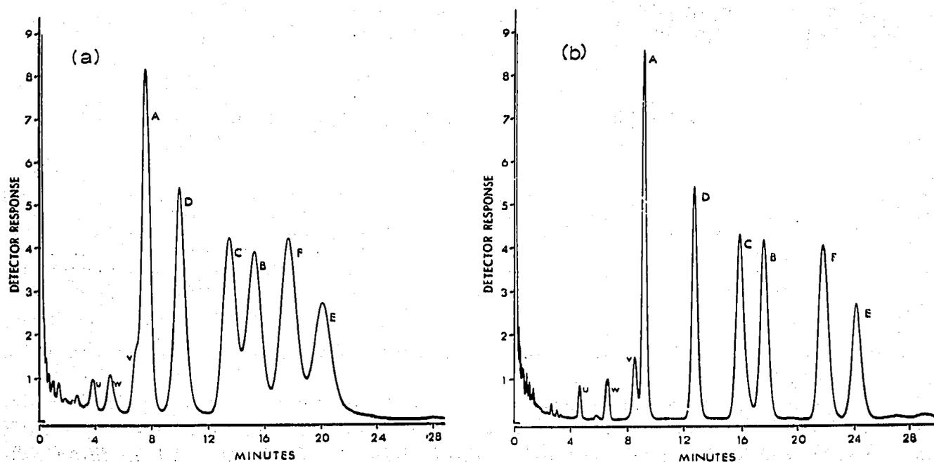
Fig. 2. Typical separations of mixed alkyl ether and monoglyceride TMS ether derivatives on non-polar liquid phases of (a) Apiezon L 240° and (b) JXR methyl silicone 225°. Peaks identified as alkyl ethers: u = C<sub>14</sub>:0; A = C<sub>16</sub>:0; v = C<sub>16</sub>:1; B = C<sub>18</sub>:0; C = C<sub>18</sub>:1 and monoglycerides: w = C<sub>14</sub>:0; D = C<sub>16</sub>:0; E = C<sub>18</sub>:0; F = C<sub>18</sub>:1.
